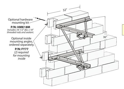
Adjustable mast offset from wall at 16", 22" and 28"
